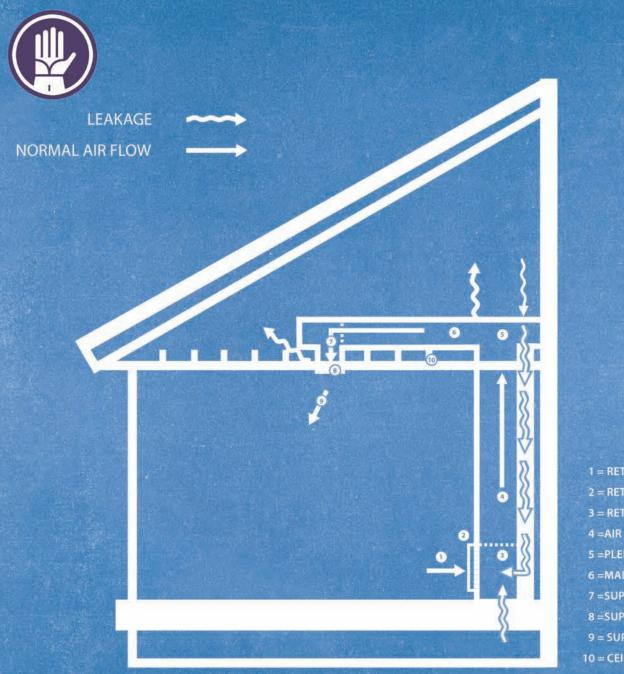
1 = RETURN AIR 2 = RETURN AIR GRILLE 3 = RETURN AIR CHAMBER 4 = AIR HANDLER 5 =PLENUM 6 =MAIN SUPPLY DUCT 7 = SUPPLY AIR DUCT 8 = SUPPLY AIR REGISTER 9 = SUPPLY / CONDITIONED AIR 10 = CEILING JOIST
